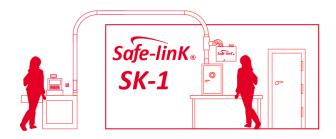
"Safe-linK" SK-1 is a one-way Air Tube system that is designed to assist cashiers in removing surplus cash from the till and delivering it directly into the safe in a secure part of the premises by vacuum. Depending on individual needs Safe-link is available in a choice of 50, 63 or 90mm diameter tubing.
