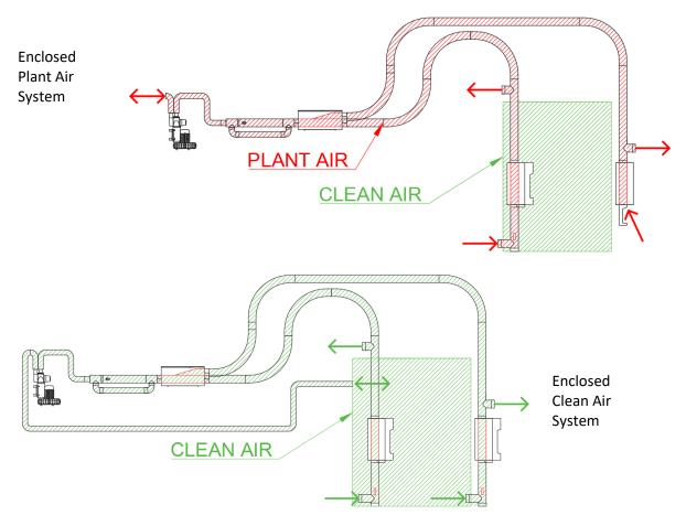
Alternatively, we can design a fully enclosed clean air system with through type stations only and tubed in clean air. Other variations are available including fine filtering air.
